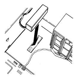
4. Connect the battery cable to connector CN1.
